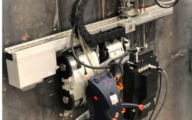
Built-in joystick controller for magwheel crawlers and XY scanners.
