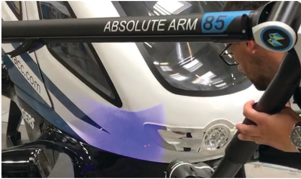
Seamless integration with market-leading 6DOF positioning devices like Hexagon's CMM arms and laser trackers for full 3D data acquisition.
