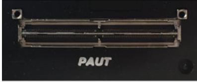
The cartridge features an I-PEX connector with standard pinout, offering PAUT probe compatibility with other brands.
